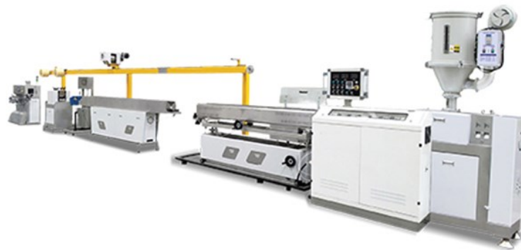
Figure 1. The extruder used to produce PLA/Nano silica filament
